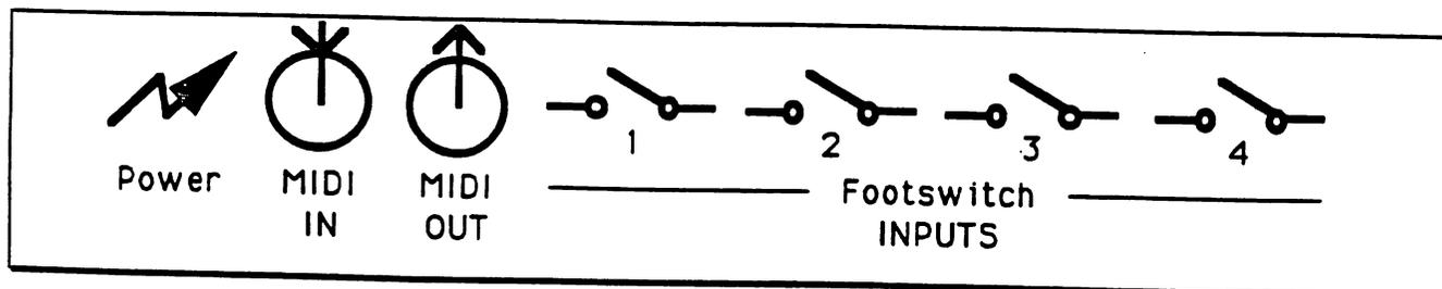
Power Supply, (9VDC / 200mA, center +) 2.1mm plug, 11.5mm barrel
