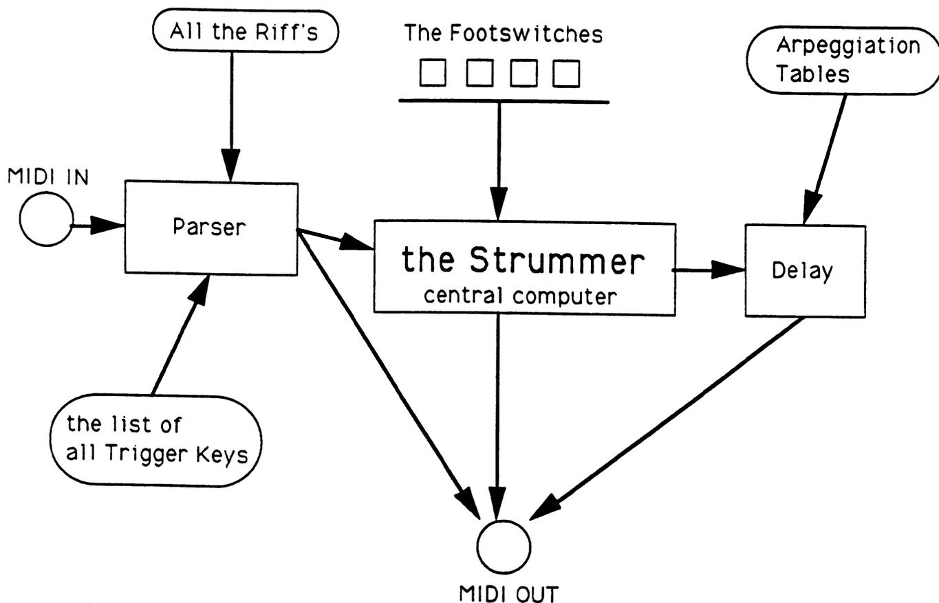
The first thing that the Strummer does when it receives a MIDI message is to look at the channel number. The Parser (the Strummer's MIDI Traffic Cop) will immediately pass any messages that aren't on the Strummer's MIDI In channel directly to the MIDI OUT.
